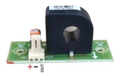
NB: If you don't need Battery current limiting, connect two 4.7K resistor to DC- CT connector (EconoMPPT board) as shown in picture.
