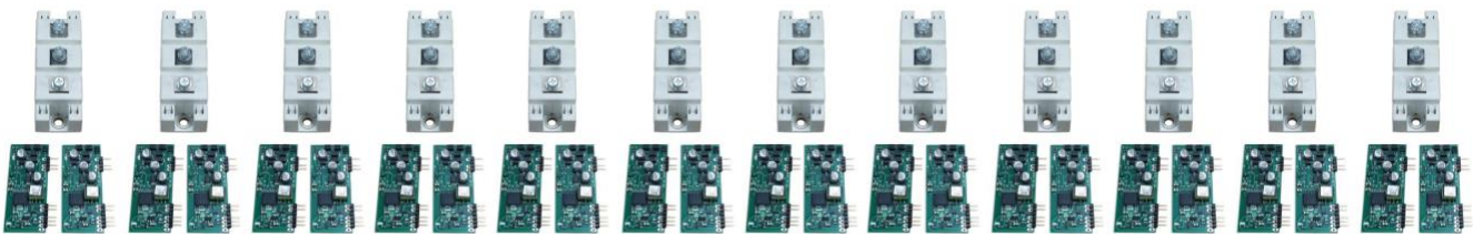
12 IGBT modules and 24 drivers used in existing Static Voltage Stabilizers including QUIKorrect for a three phase stabilizer
