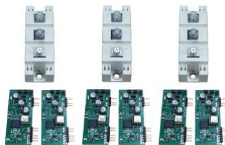
In TrioStat, only 3 IGBT modules and 6 drivers are enough for a three phase stabilizer
