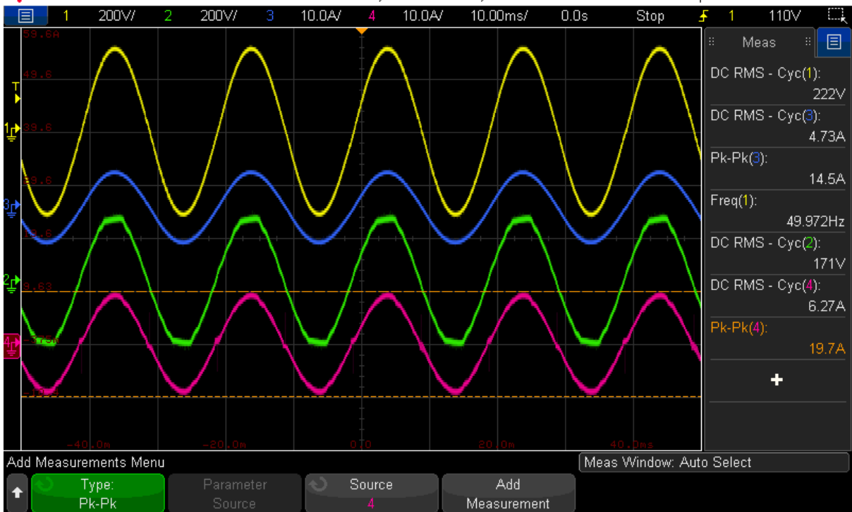
Figure 7 – Yellow output voltage, blue output current, green input voltage, red input current
